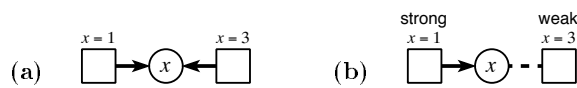
Fig. 2. (a) A solution graph for an over-constrained system and (b) one for a constraint hierarchy
