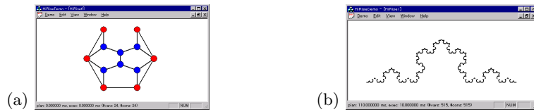
Fig. 1. Sample applications of HiRise: (a) one that allows a user to edit a graph by adding, moving, and staying nodes, and fixing edge directions, where each inner node is constrained at the barycenter of its adjacent nodes; (b) another that enables a user to operate a picture that approximates the fractal diagram known as the Koch curve, which is realized with a finite number of vertices constrained by linear equations
